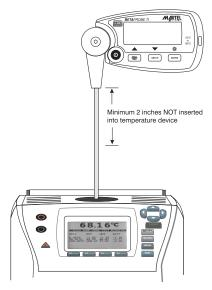
For best results, allow ample time for the probe to stabilize before recording measurements. The stability display is helpful for this.
